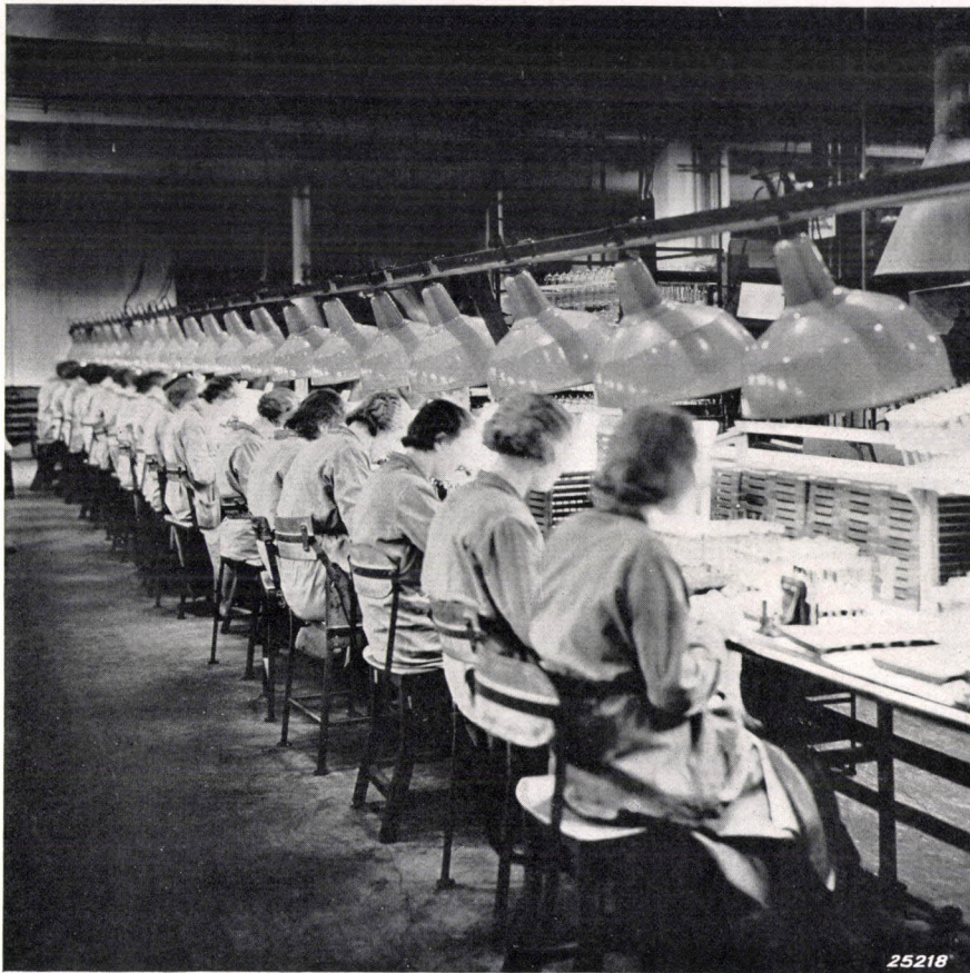
Fig. 4. Work-bench in an assembly department with the illumination whose results are shown in figs. 3a) and b).
