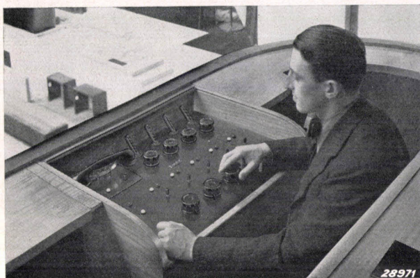
Fig. 3. Poste de régie in the "Salle des Assemblées". At the front of the control table may be seen the knobs for regulating the potentiometers R , and at the upper right-hand side the four switches for regulating the sound intensity of the loud speakers. Above these are the neon indicators which indicate the sound intensity at different spots in the hall (see the last section: signaling).
